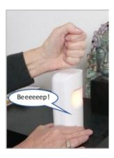
Continuously tap or shake the sensor firmly (to activate the vibration sensor) and wait until it beeps and the light turns red.
